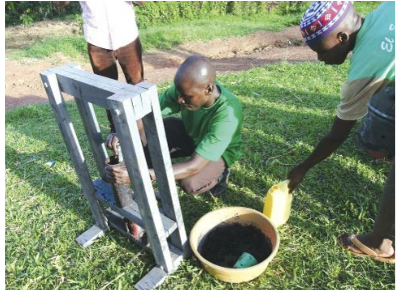
Waste residues are placed in the molding machine and pressed to make charcoal briquettes
