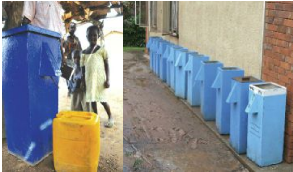
A bio-sand filter in use (photograph: www.water.org ) and more waiting to be collected outside A Rocha Uganda's Kampala office
