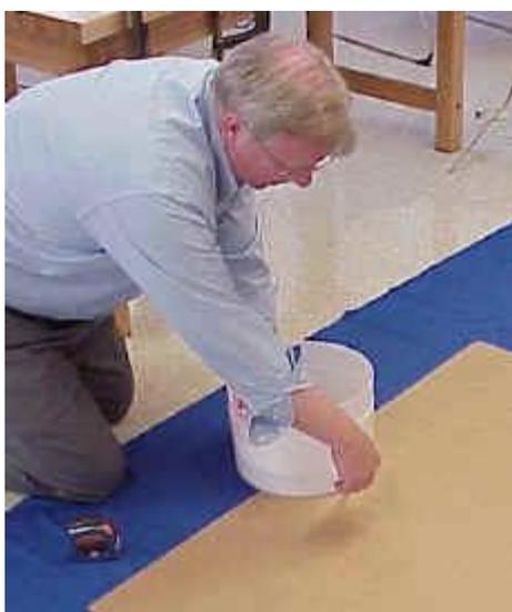
Cut a half circle out of the cardboard, along the bottom. When the funnel is formed, this becomes a full-circle and should be wide enough to go around your cooking pot. So for a 18cm diameter cooking pot, the radius of the half-circle is 18cm. For a litre canning jar, cut a 13cm radius half-circle out of the cardboard.
