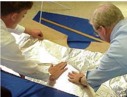
Apply glue or adhesive to the top (inner) surface of the cardboard, then quickly apply the aluminium foil on top of the glue, to affix the foil to the cardboard. Make sure the shiniest side of the foil is on top, since this becomes your reflective surface in the funnel. Put just enough glue for one width of foil, so that the glue stays
